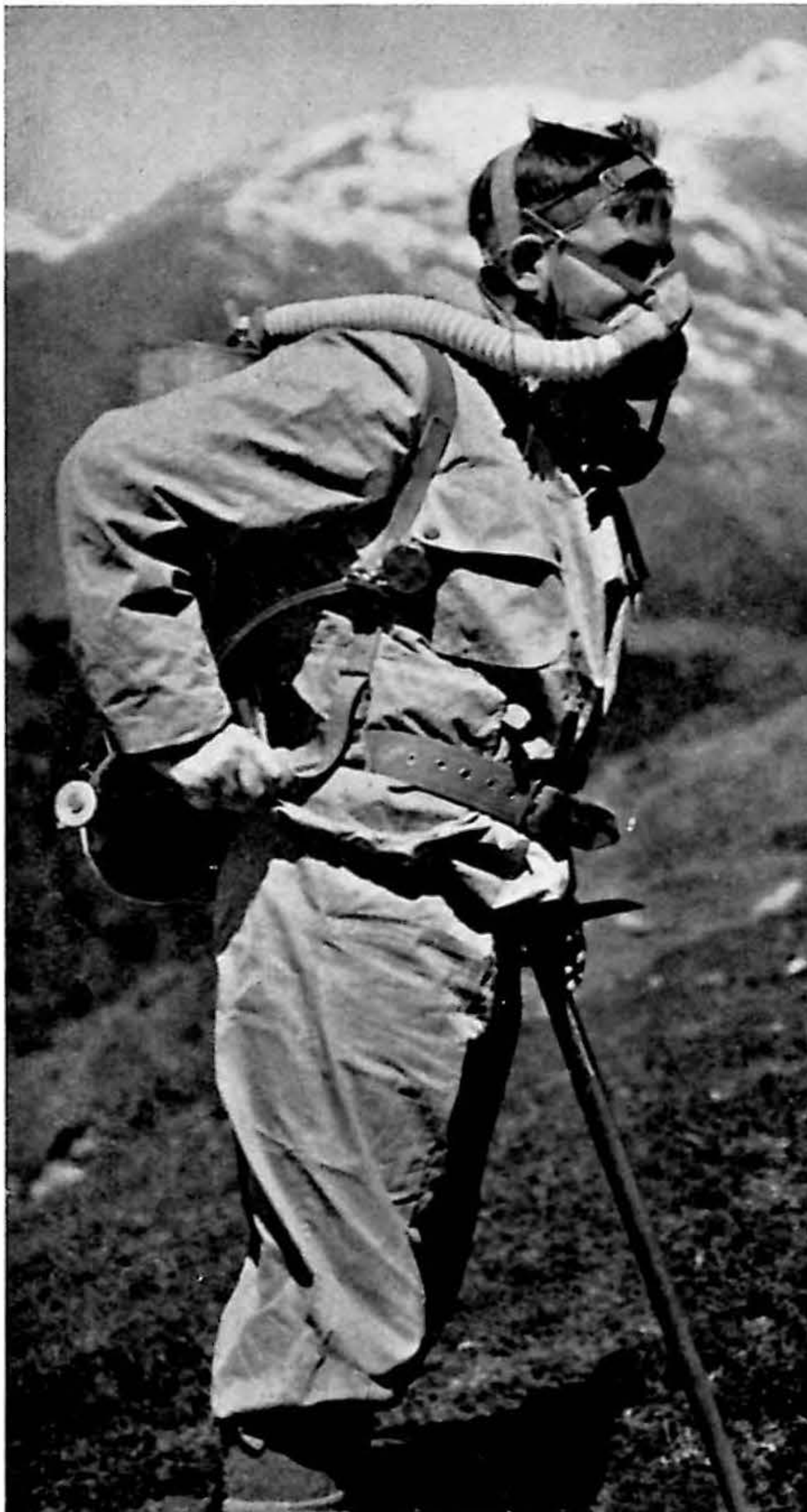
RE-BREATHING TYPE OF OXYGEN APPARATUS. Reproduced by the courtesy of the Editor, Geographical Journal .
